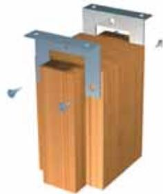
Ensuring that the post is plumb, place the TS500B bracket onto the underside of the upright post and the face of the base section. Fix into position using a wafer head screw.
